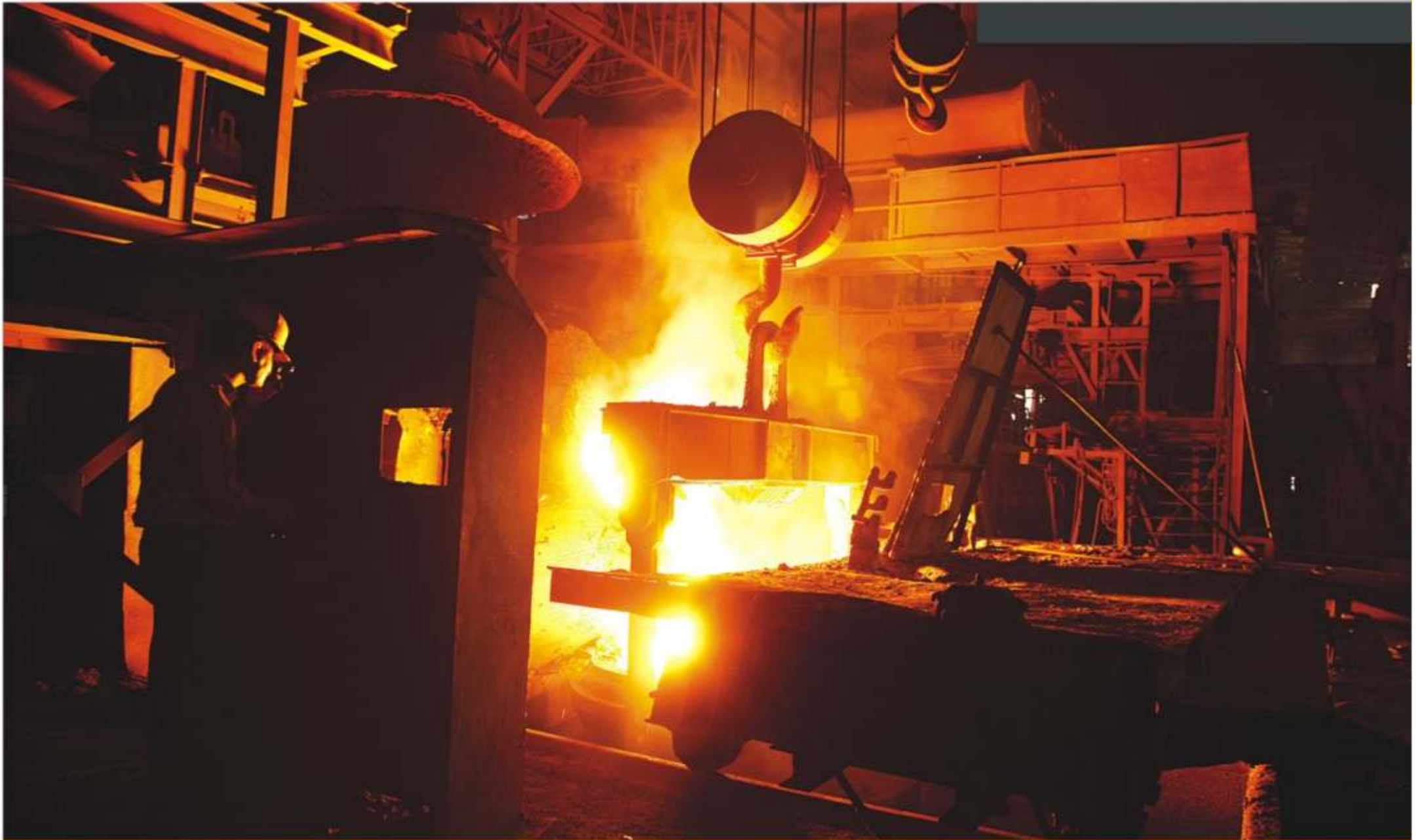
Tapping of liquid stainless steel from AOD at Facor Steels Limited, Nagpur
