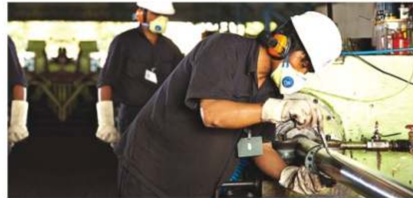
Bright Bar Inspection at Facor Steels Ltd., Nagpur
